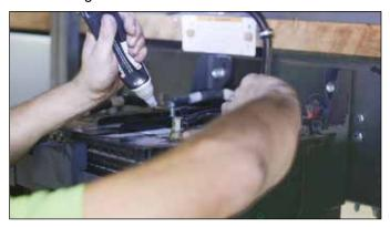
17. Replace the battery box cover and lock it in place.
