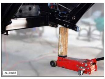
4. Determine the installed height (B) of the adapter frame tube using the charts and the illustration.
