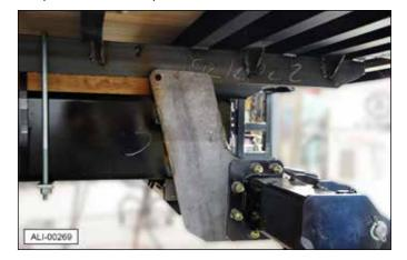
21. Remove the installation brackets from the floor extension.
