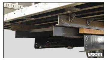
**Note:** Walk ramp stops may need to be removed. If the walk ramp is equipped with cage wheels, and they are removed, fill the open cut-outs as shown below to ensure a smooth walk ramp function.
