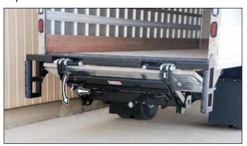
SAFETY INSTRUCTIONS When placing the liftgate in the storage position (folding), slowly fold the platform until it contacts
