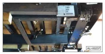
**Important:** Make sure the walk ramp cage does not hang below the walk ramp support box.
