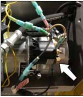
For gravity-down models, simply press and hold the control switch in the DOWN position to release the pressure in the cylinder.
