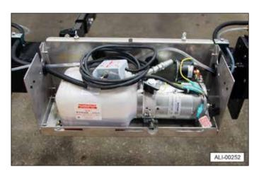
**Note:** The power unit box should contain the power cable and switch, plastic tie wraps for the battery cable, and one package containing decals, shims, a 200 Amp fuse, and manuals.
