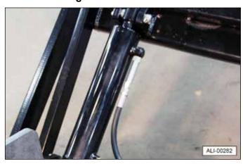
If the cylinder does not operate or operates slower than normal, remove the flow control valve and hook the hydraulic hose directly to the cylinder. If the cylinder operates properly, replace the flow control valve.
