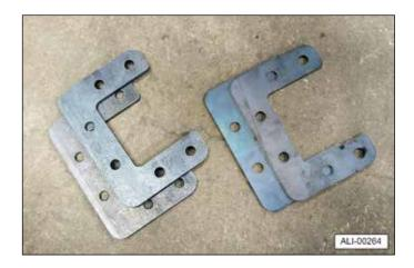
To adjust the width, remove the six bolts and nuts from each mounting plate. Add or remove spacers to achieve the desired width, and replace the bolts and nuts. Be sure to make the same adjustment on both sides to keep the liftgate centered.
