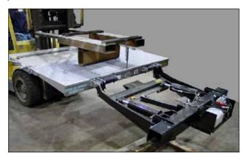
This lifting device must be made specifically for the type and design of the particular forklift used in the installation. Remember, the materials used to construct the lifting device must be capable of lifting and supporting the liftgate being installed. The lifting device must also contain a retaining method to hold it onto the forklift.
