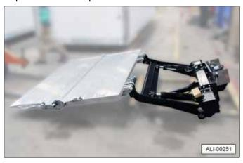
**Note:** A spacing guide is installed over the end of the cylinder rod. Do not remove this guide until the liftgate has been tack welded in place on the truck body.
