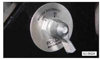
Cut-Off Switch Mounted in Cab of Truck.
